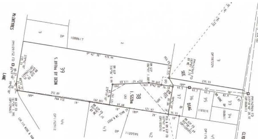
Figure 2 – Subdivision layout as approved by DA1996/1037. Lot 38 contains the restriction marked (A) and Lot 39 is now the subject of the current proposed subdivision.
