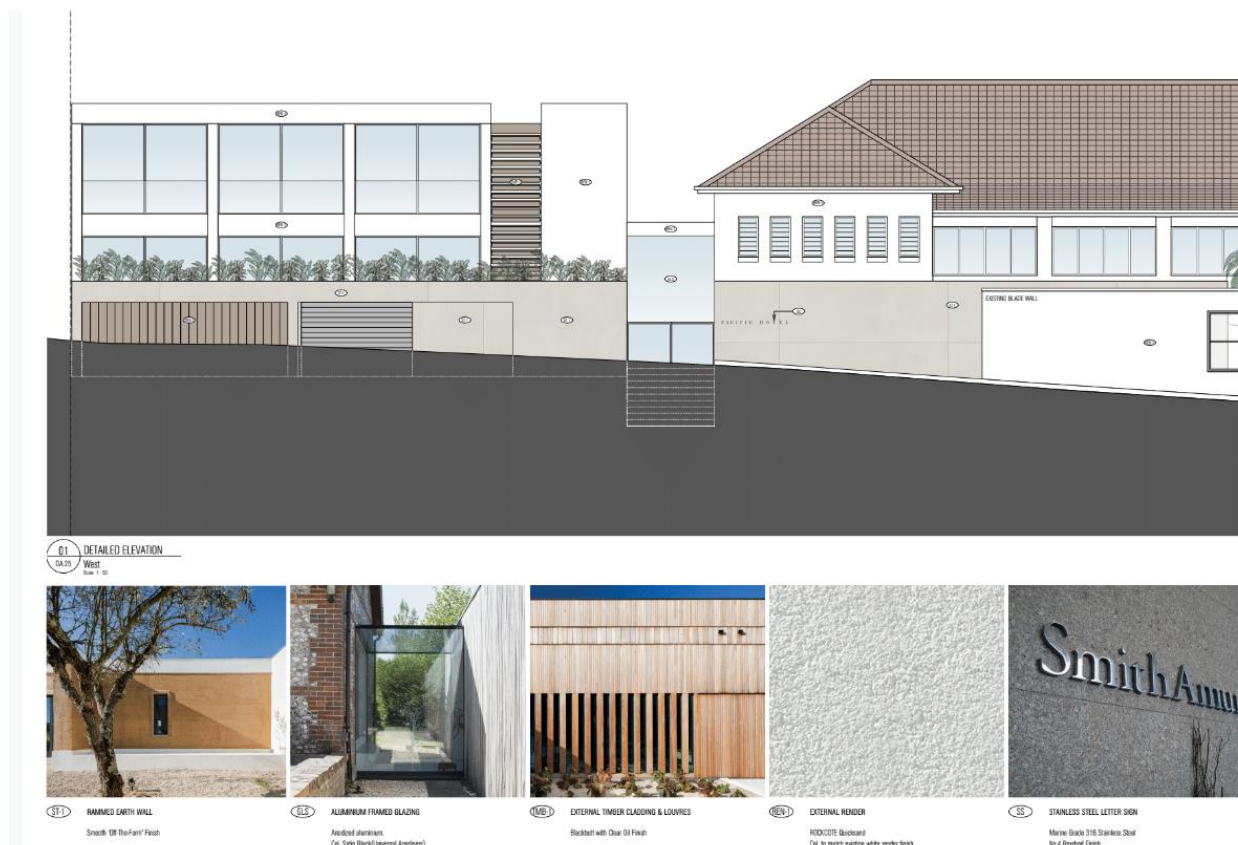
Figure 5 – Detailed west elevation of the proposed development with samples of proposed external surface treatments.
