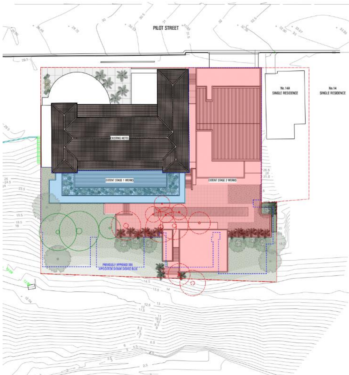
Figure 2 – Site plan extract showing proposed Stage 1 (blue) and 2 (pink) works as well as extent of works approved in 2013 (blue dashed line).
