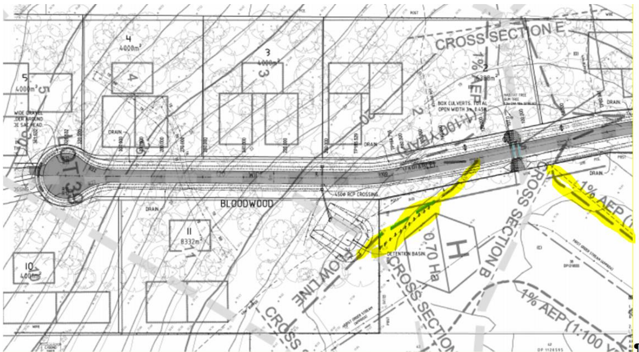
Diagram 1 – overlay showing differences in flow lines on adjoining Lot 38 between the two assessments and proximity to detention basin
