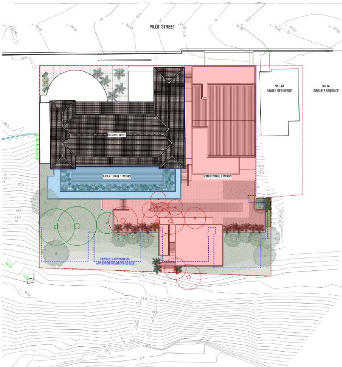
Figure 2 – Site plan extract showing proposed Stage 1 (blue) and Stage 2 (pink) works as well as extent of works approved in 2013 (blue dashed line).
