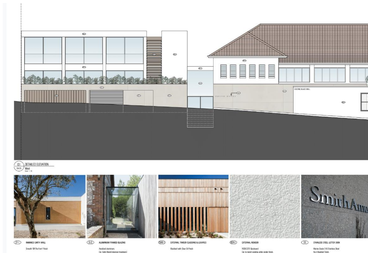
Figure 5 – Detailed west elevation of the proposed development with samples of proposed external surface treatments.
