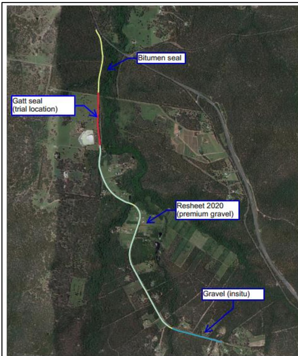
Figure 6: Dinjerra Road showing works conducted since 2019
