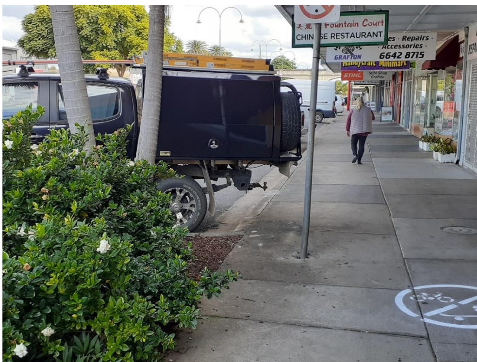
Plate 2 – Reverse parked 4WD vehicle in Prince Street, Grafton showing significant overhang to footpath even though vehicle has stopped short of kerb.
