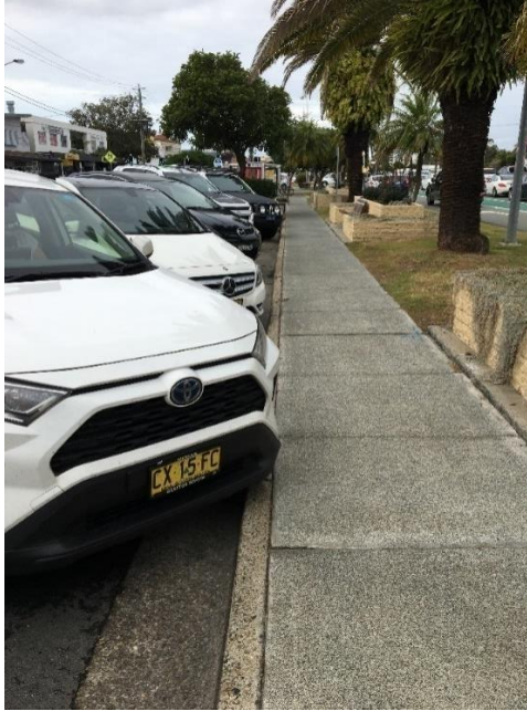
Plate 1 - Nose-in parking adjacent to a pedestrian footpath in Tugun, QLD showing the relatively small (or no) overhang from vehicles including a 4WD (5 th vehicle from front).
