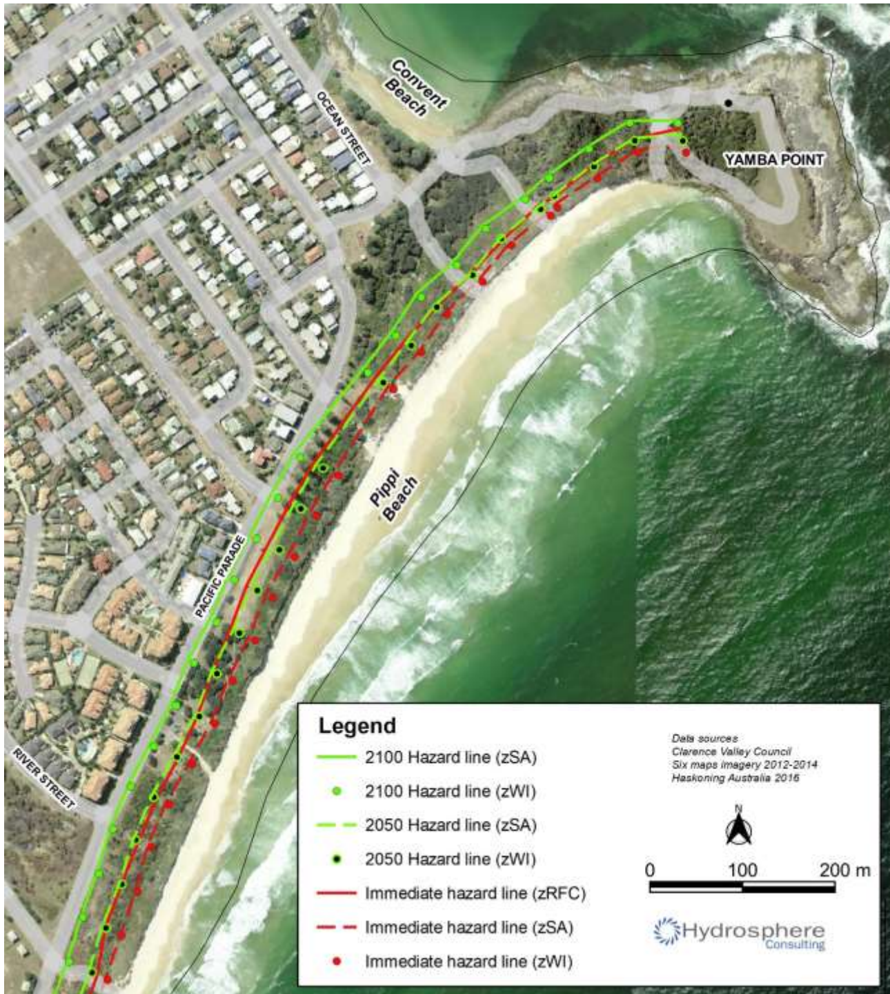
Figure 25: Coastal hazard lines for Pippi Beach - north
