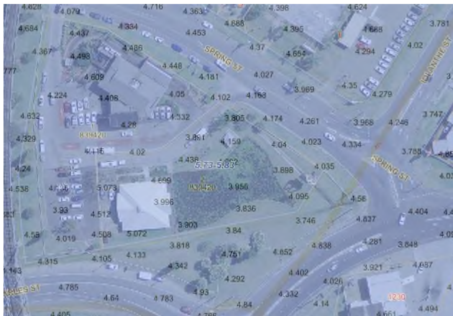
Ground Levels on the site
