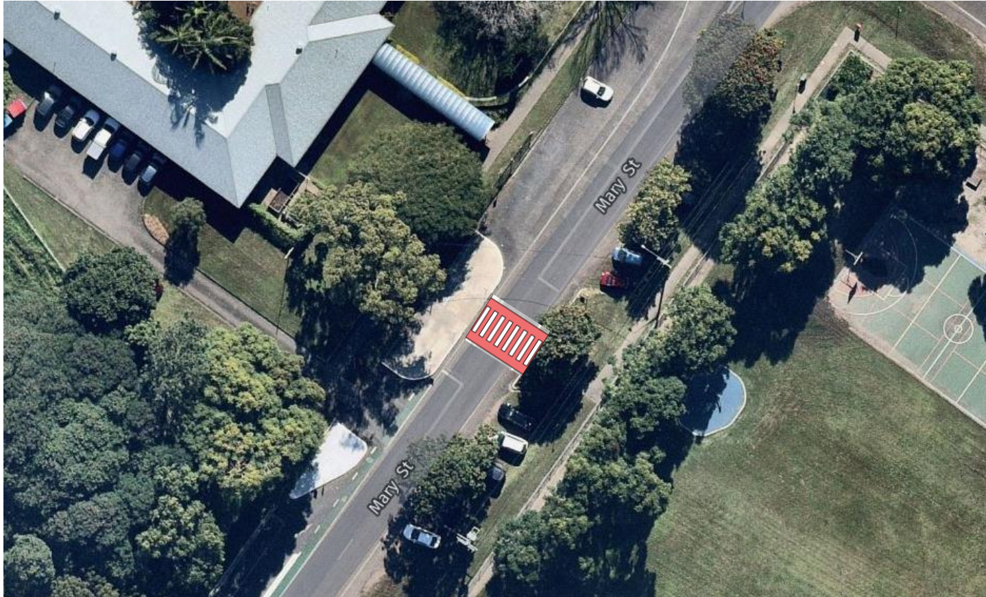
Upgrade Childrens Crossing to Combined Pedestrian and Childrens Crossing in Mary Street between Grafton Infants and Public School.
