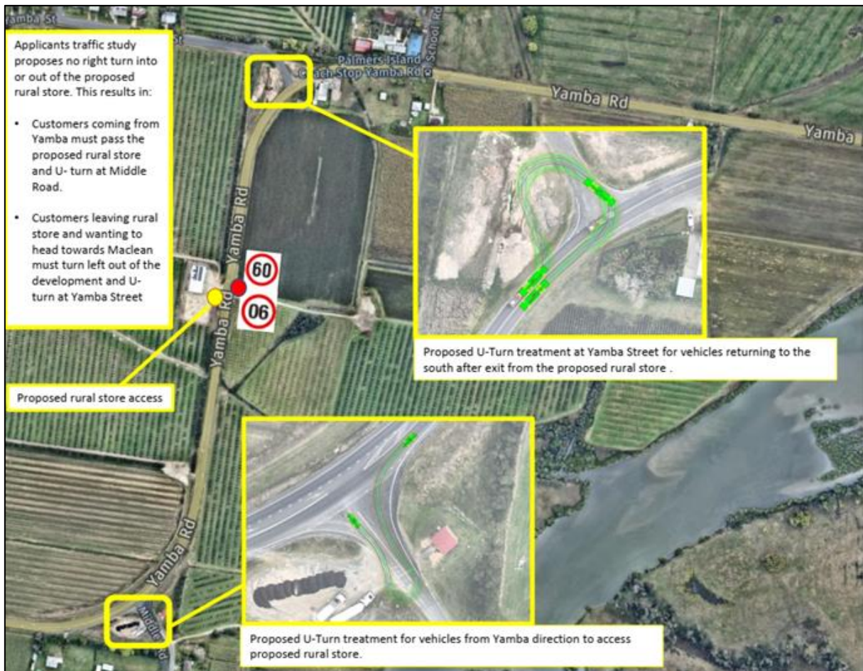
Figure 5: Proposed U-turn treatments showing proposed rural store access and current speed zones
