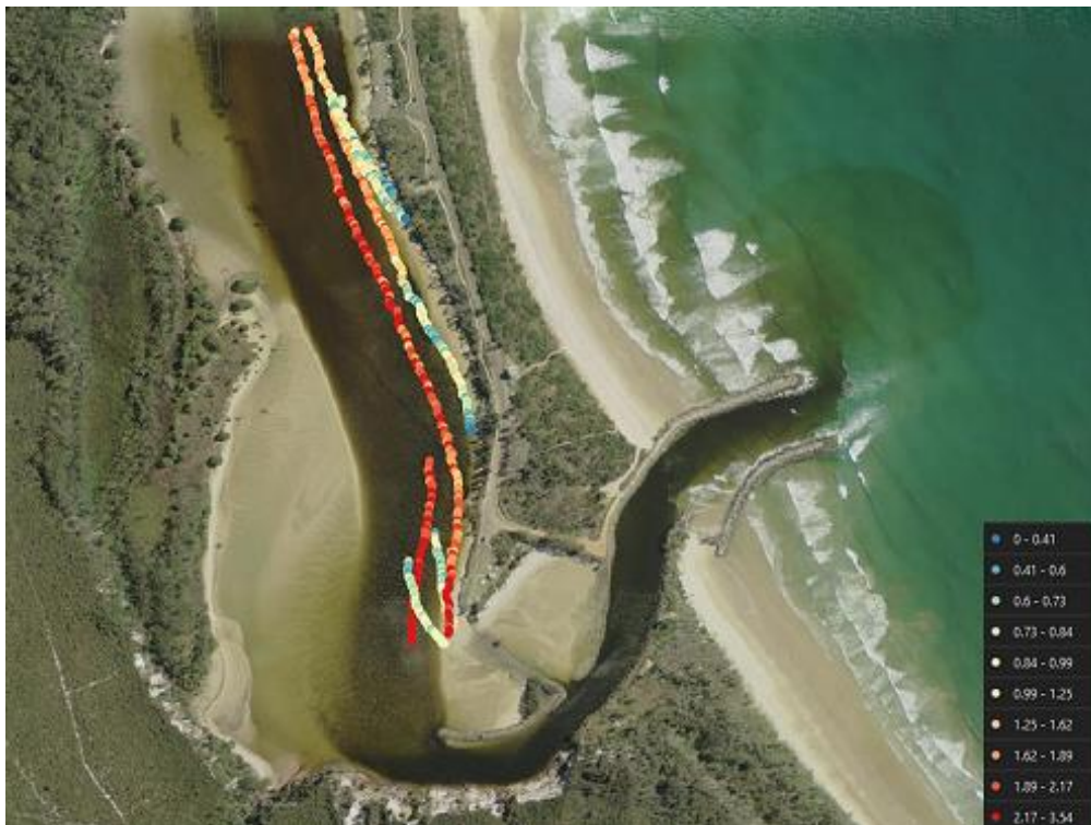
Figure 2-22: Recorded tidal current velocity near the Wooli Wooli River entrance
