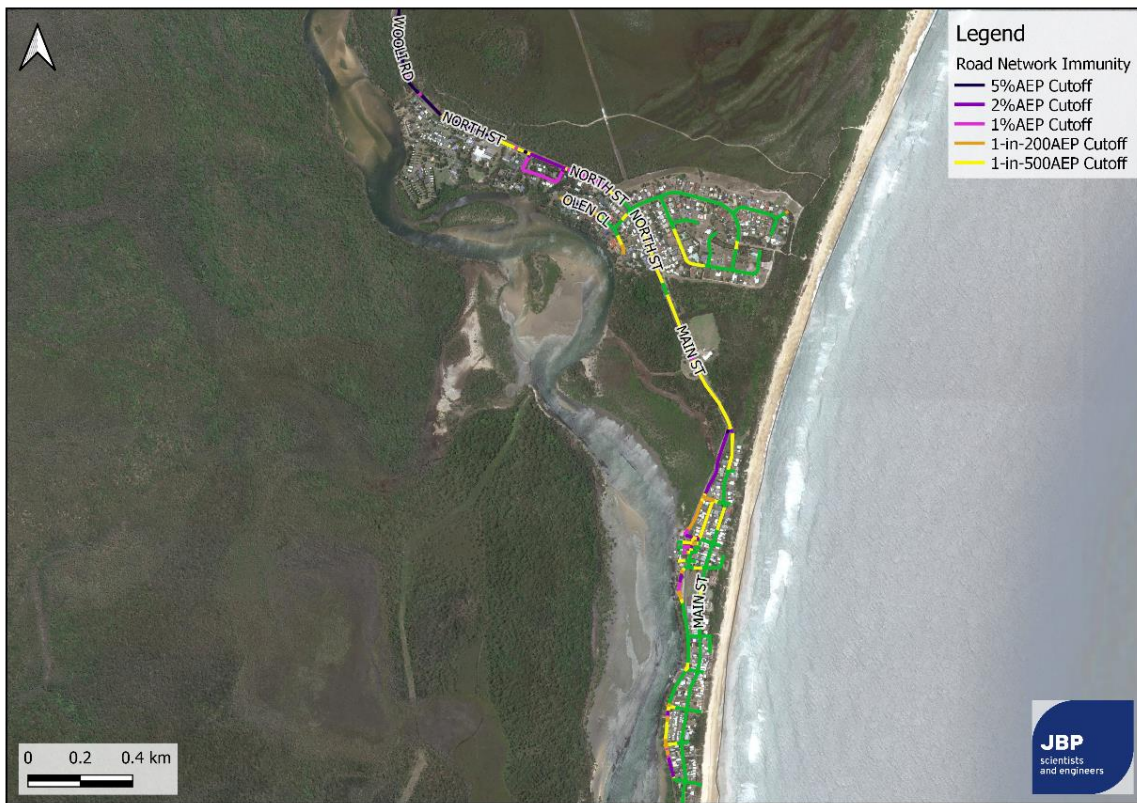
Figure 6-3. Road network evaluation examples showing network trafficability and duration of closure information.
