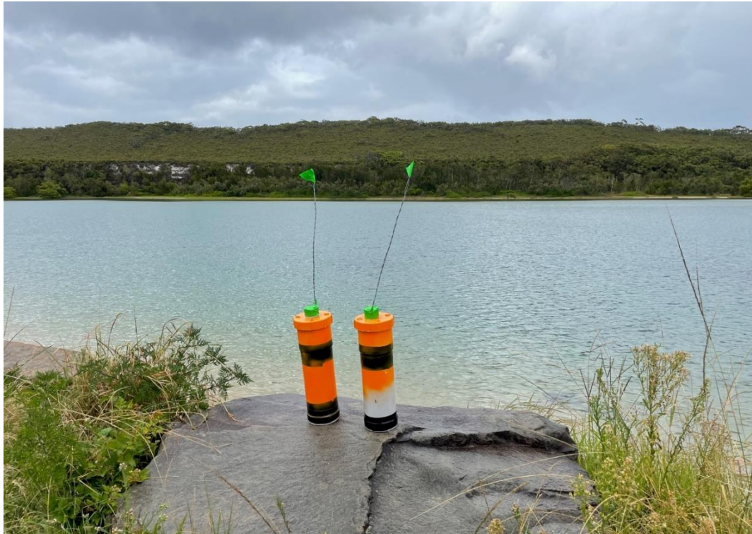
Figure 2-21: Drifter technology used to measure tidal current velocity
