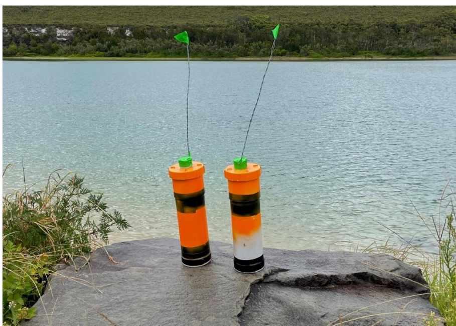
Figure B-4: Drifter instrumentation used during Wooli Wooli River current speed investigation
