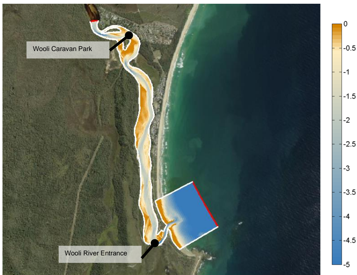
Figure B-2: Computational grid extent and bathymetry for Delft3D model, open boundaries shown in red.
